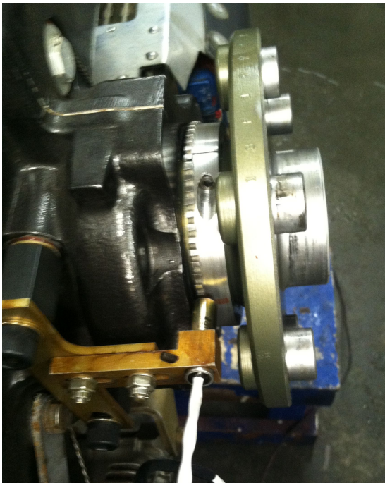
Figure 5: Components that make up the Lycoming CSTW Sensor Bracket; 1. Pick-Up Bracket; 2. Pick-Up Holder; 3. Magnetic Pick-up (Magnetic Sensor); hardware is not shown for clarity.
