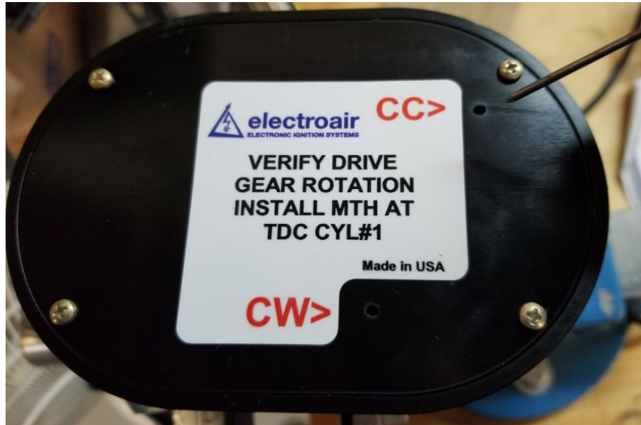
Figure 10: Installation of MTH Alignment Pin
