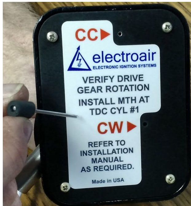
Figure 7: Installation of MTH Alignment Pin
